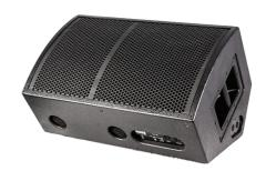
The enclosure houses a reflex-loaded 4" (102mm) voice coil, 12" (305mm) waterproofed neodymium cone driver, matched via a signature EM Acoustics passive crossover to a 3" (76mm) diaphragm, 1.4" (36mm) exit neodymium HF compression driver coupled to a variable dispersion waveguide. This waveguide produces a coverage pattern of 90°H x 40°V at one metre, narrowing to 50°H x 40°V at three metres. This pattern gives a performer freedom of movement whilst minimizing spill into adjacent microphones.
